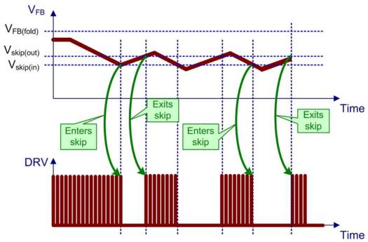
Figure 58. Skip Mode Timing Diagram
