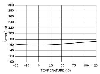
Figure 41. Fault Timer Duration t<sub>fault</sub>
