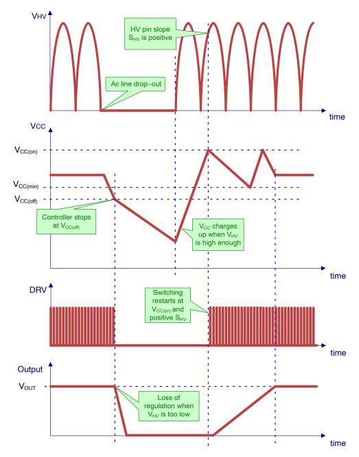
Figure 47. Ac Line Drop-out Timing Diagram
