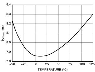
Figure 22. Maximum ON Time  $t_{\mbox{ONmax}}$  for the 100 kHz Version
