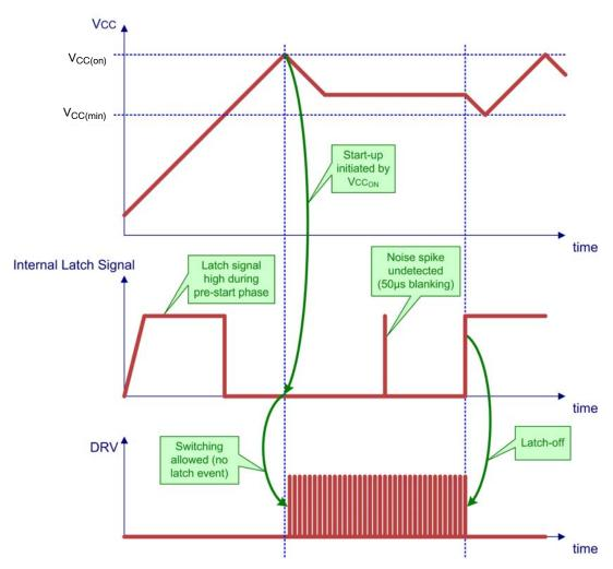
Figure 70. Latch Timing Diagram
