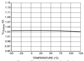
Figure 9. Threshold for Immediate Fault Protection Activation  $V_{CS(stop)}$
