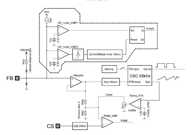
Figure 60. Slope Compensation Block Diagram
