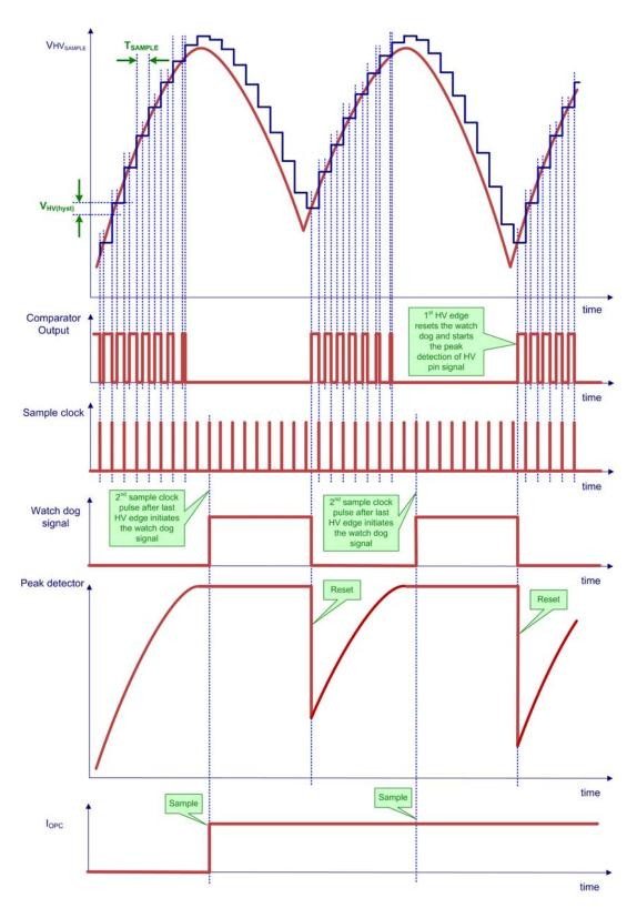
Figure 66. Overpower Compensation Timing Diagram
