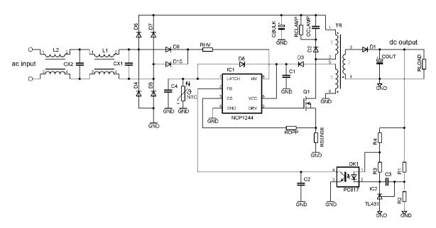
Figure 1. Flyback Converter Application Using the NCP1244
