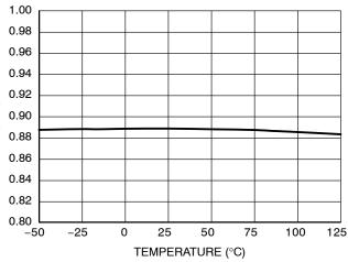
Figure 26. FB Pin Voltage Below Which Frequency Foldback Complete V<sub>FB(foldE)</sub>
