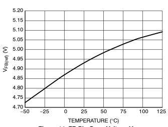
Figure 14. FB Pin Open Voltage V<sub>FB(ref)</sub>
