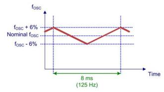
Figure 55. Frequency Modulation of the Maximum Switching Frequency
