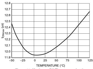
Figure 21. Maximum ON Time t<sub>ONmax</sub> for the 65 kHz Version
