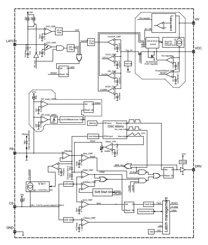
Figure 2. Simplified Internal Block Schematic
