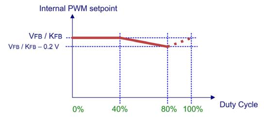
Figure 61. Slope Compensation Timing Diagram
