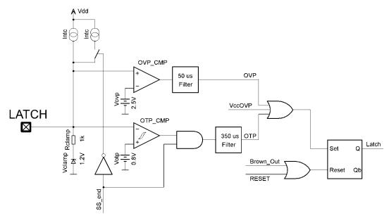
Figure 69. Latch Detection Schematic
