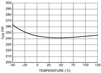
Figure 11. Leading Edge Blanking Duaration  $t_{\text{LEB}}$
