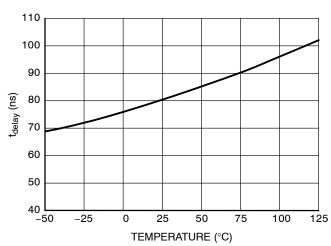
Figure 10. Propagation Delay t<sub>delay</sub>
