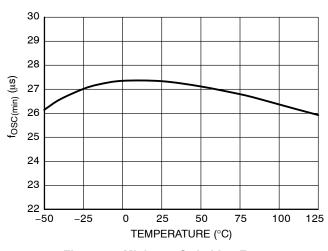
Figure 24. Minimum Switching Frequency f<sub>OSC(min)</sub>
