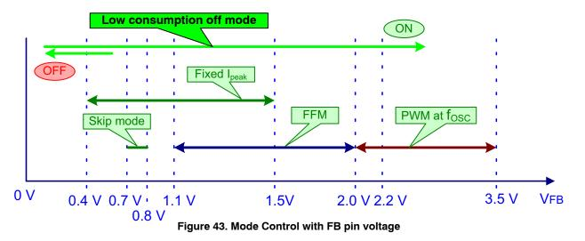
There was implemented the low consumption off mode allowing to reach extremely low no load input power. This mode is controlled by the FB pin and allows the remote control (or secondary side control) of the power supply shut—down. Most of the device internal circuitry is unbiased in the low consumption off mode. Only the FB pin control circuitry and X2 cap discharging circuitry is operating in the low consumption off mode. If the voltage at feedback pin
