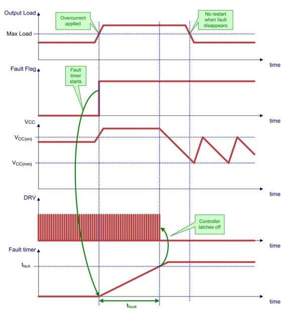
Figure 67. Latched Timer-Based Overcurrent Protection (Option A)
