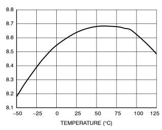
Figure 6. High Voltage Startup Current Flowing Out of  $V_{CC}$  Pin  $I_{start2}$
