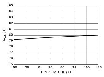
Figure 23. Maximum Duty Ratio D<sub>MAX</sub>
