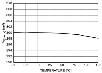
Figure 8. Frozen Current Setpoint  $V_{l(freeze)}$  for the Light Load Operation
