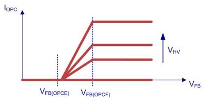
Figure 63. Overpower Protection Current Relation to Feedback Voltage
