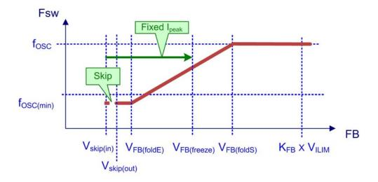
Figure 56. Frequency Foldback Mode Characteristic
