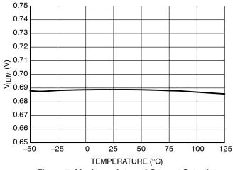
Figure 7. Maximum Internal Current Setpoint  $V_{\text{ILIM}}$
