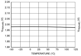
Figure 25. FB Pin Voltage Below Which Frequency Foldback Starts V<sub>FB(foldS)</sub>
