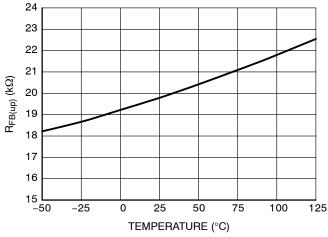
Figure 13. FB Pin Internal Pull-up Resistor R<sub>FB(up)</sub>
