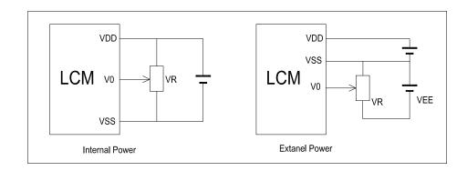
$V_{DD^{\sim}}V_0\text{: LCD Driving voltage}$
