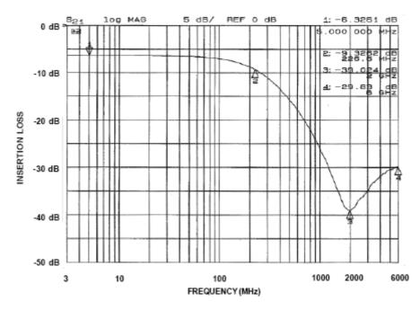
Typical Filter Performance (T<sub>A</sub> = 25°C, DC Bias = 0 V, 50  $\Omega$  Environment)
