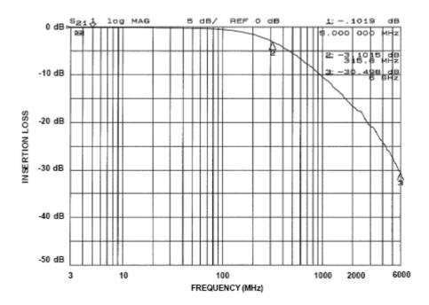
Figure 4. Insertion Loss vs. Frequency, Filter 4 (Pins 4 and 5)
