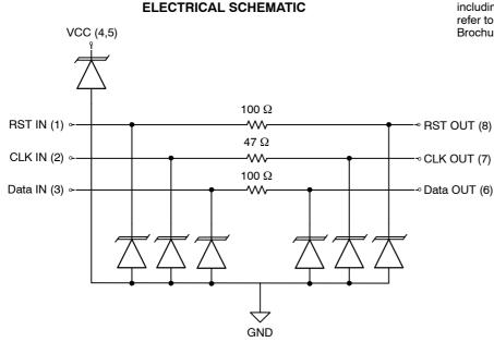
\*See Package/Pinout Diagrams for expanded pin information.
