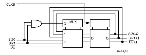
Figure 3. Logic Diagrams for SIZ0, SIZ1, and **BE** Register
