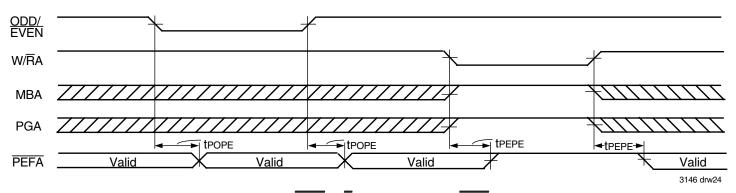
Figure 24. ODD/EVEN. W/RA, MBA, and PGA to PEFA Timing
