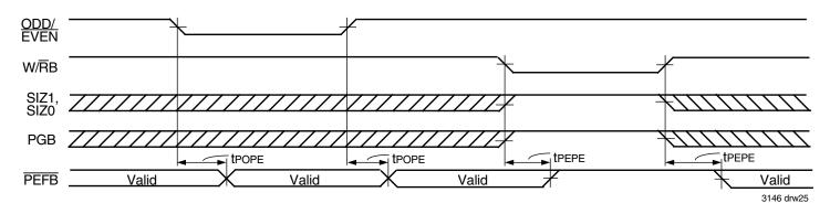
Figure 25. ODD/EVEN. W/RB, SIZ1, SIZ0, and PGB to PEFB Timing
