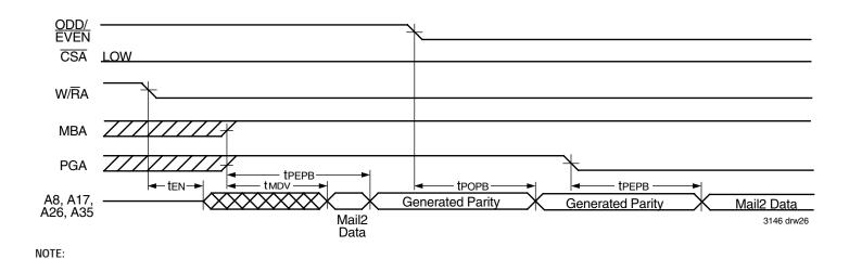
Figure 26. Parity Generation Timing when Reading from the Mail2 Register
