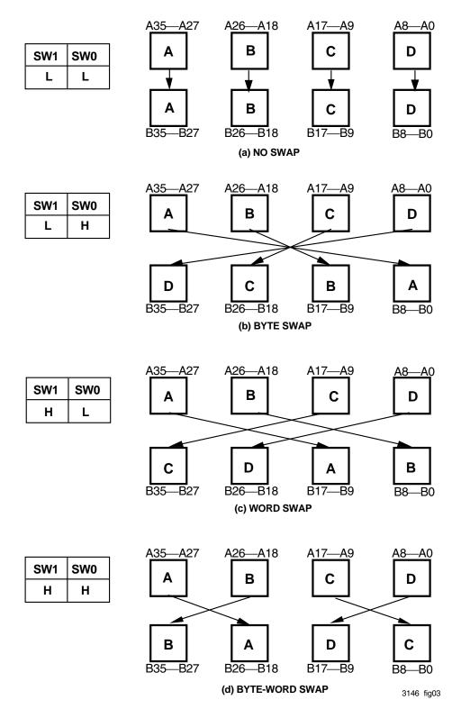
Figure 4. Byte Swapping (Long Word Size Example)
