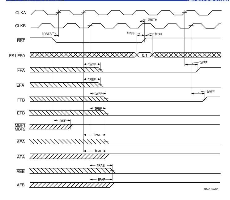
Figure 5. Device Reset Loading the X Register with the Value of Eight
