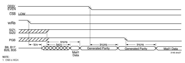
Figure 27. Parity Generation Timing when Reading from the Mail1 Register
