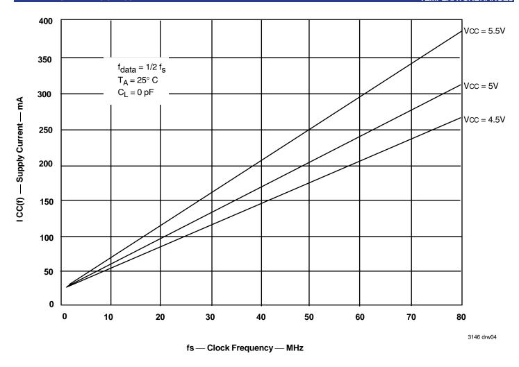
Figure 1. Typical Characteristics: Supply Current vs Clock Frequency
