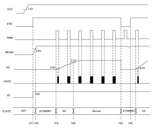
Figure 32. PWM Start up 1 (Input PWM Signal After Input STB Signal)
