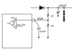
Figure 27. OVP setting example
