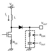
Output capacitor needs to be selected in consideration of equivalent series resistance
