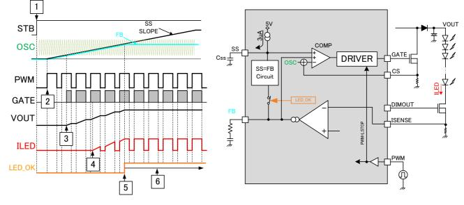
Figure 20. Startup waveform
