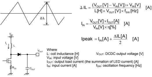
Figure 29. Inductor current waveform and diagram
