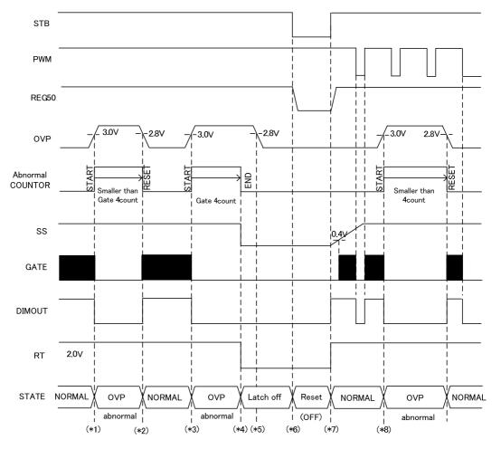
Figure 36. OVP Detection
