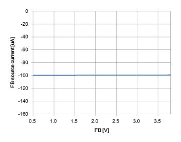
Figure 10. FB source current vs FB voltage characteristic
