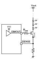
Figure 15. DIMOUT terminal circuit example
