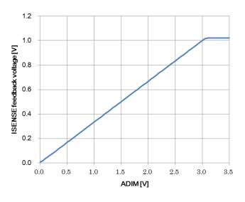
Figure 11. ISENSE feedback voltage vs ADIM voltage characteristic
