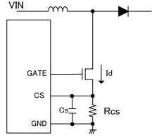
Figure 16. CS terminal circuit example
