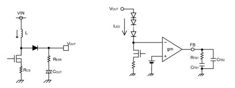
Figure 31. Output stage and error amplifier diagram
