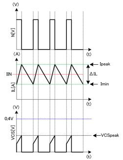
Figure 28. Coil current waveform
