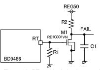
Figure 12. RT terminal circuit example
