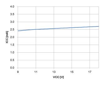
Figure 7. Circuit current (active)
