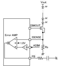
Figure 14. ISENSE terminal circuit example
