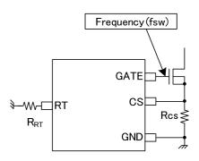
Figure 25. RT terminal setting example
