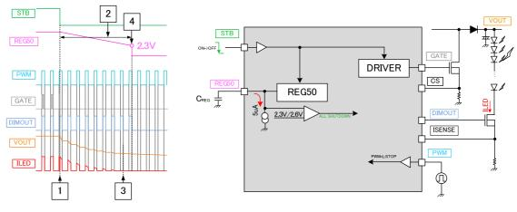
Figure 22. The waveform and diagram at shutdown
