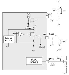
Figure 23. VCC series resistance circuit example
