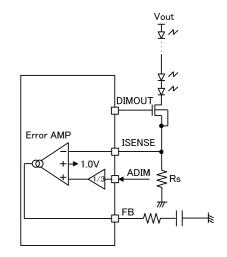
Figure 24. LED current setting example
