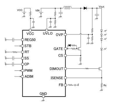
Figure 17. Basic application example
