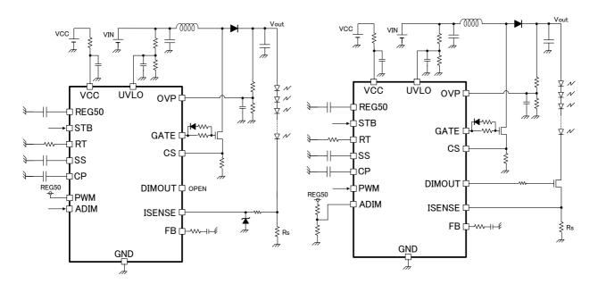
Figure 18. Example circuit for analog dimming
