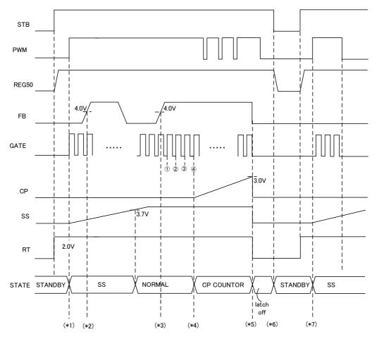
Figure 37. FBMAX Detection
