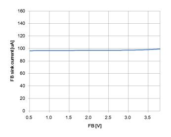
Figure 9. FB sink current vs FB voltage characteristic
