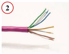
Untwist the pairs and Straighten the Wires
