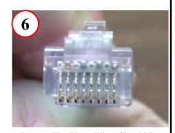
Inspect The Plug; Wires Should Be Visible from Plug Front
