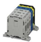
High-current terminal block, Connection method: Screw connection, Number of positions: 5, Cross section: 16 mm<sup>2</sup> - 95 mm<sup>2</sup>, AWG: 4 - 3/0, Width: 101.5 mm, Height: 80 mm, Color: gray/blue/black-yellow, Mounting type: ct screw connection
