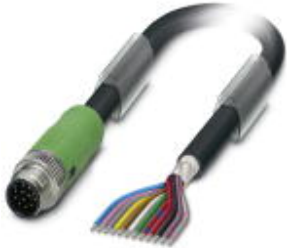
Sensor/Actuator cable, 12-position, PUR/PVC, Black RAL 9005, shielded, Plug straight M12 SPEEDCON, A-coded, on free cable end, Cable length: 10 m
