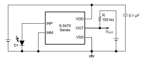
Figure 21 Example Certain Photocurrent Level Detector (Nch Open-drain Output Product)
