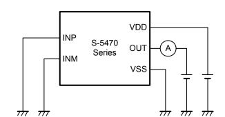
Figure 10 Test Circuit 6
