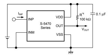
\*1. Resistor (R) is unnecessary for the CMOS output product.
