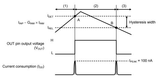
Figure 16 Operation when Detecting the Difference of Current Level
