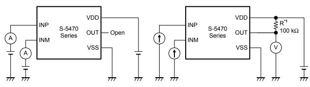
1. Resistor (R) is unnecessary for the CMOS output product.
