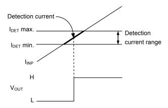
Figure 18 Detection Current
