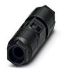
Conductor connectors, QUICKON connection, No. of pos.: 3+PE, 0.5 mm<sup>2</sup> ... 1.5 mm<sup>2</sup>, 690 V, 17.5 A, black, With two QUICKON nuts, Cable diameter: 4 mm ... 9 mm
