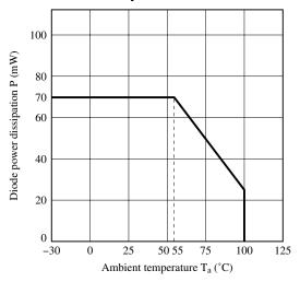
Fig.4 Total Power Dissipation vs. Ambient Temperature
