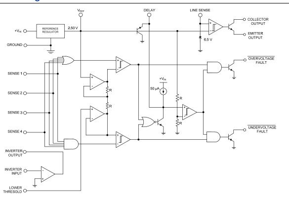
Figure 1 - Block Diagram
