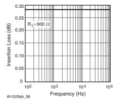
Fig. 7 - Insertion Loss vs. Frequency
