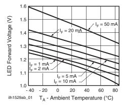
Fig. 2 - LED Voltage vs. Temperature
