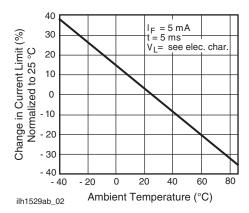
Fig. 3 - Current Limit vs. Temperature
