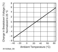
Fig. 10 - Switch Breakdown Voltage vs. Temperature
