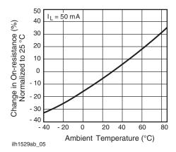
Fig. 6 - On-Resistance vs. Temperature
