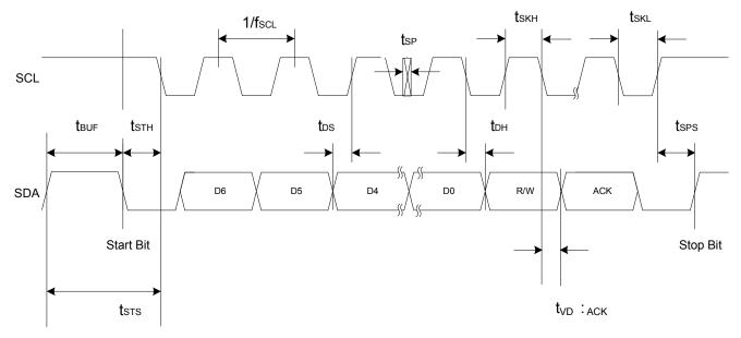
Figure 1. I<sup>2</sup>C Interface Timing Diagram
