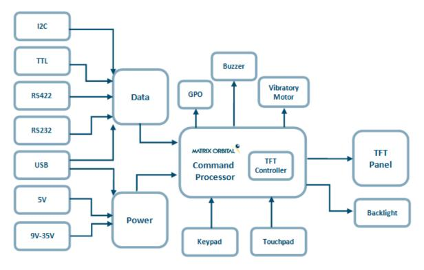
Figure 2: Functional Diagram
