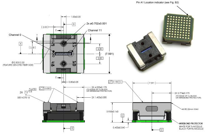
Figure 1. Module Top and Side View
