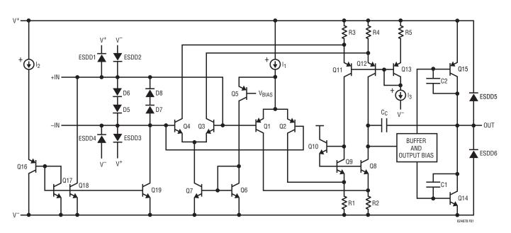
Figure 1. LTC6246/LTC6247/LTC6248 Simplified Schematic Diagram
