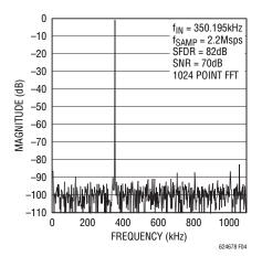
Figure 4. 350kHz FFT Showing 82dB SFDR
