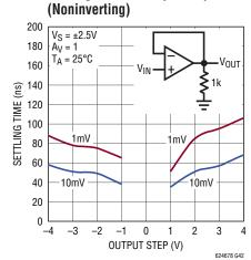
**Settling Time vs Output Step**
