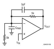
Figure 2. 5pF Feedback Cancels Parasitic Pole
