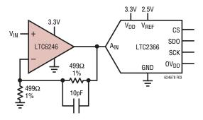
Figure 3. Single Supply 12-Bit ADC Driver
