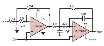
Figure 8. Single 2.7V Supply 4MHz 4th Order Butterworth Filter
