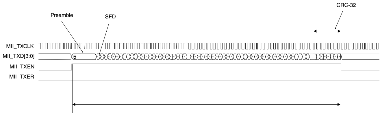
Figure 11-26. MII transmit operation
