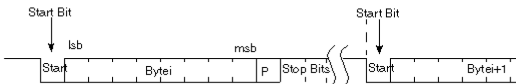
Figure 11-44. Start Bit Diagram
