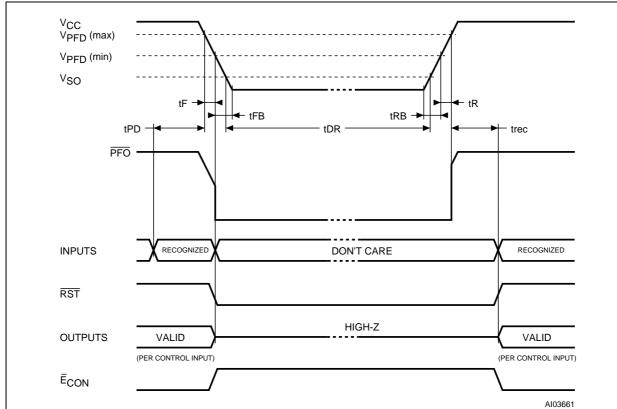
Figure 22. Power Down/Up Mode AC Waveforms
