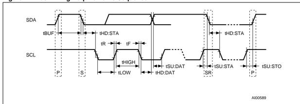
Figure 21. Bus Timing Requirements Sequence
