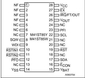
Note: No Function (NF) pins should be tied to V<sub>SS</sub>. Pins 1, 2, 3, and 4 are internally shorted together.
