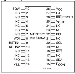
Figure 5. 28-pin, 300mil SOIC (MX) Connections
