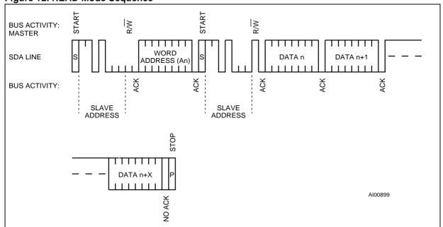
Figure 13. Alternate READ Mode Sequence
