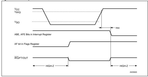
Figure 18. Back-Up Mode Alarm Waveform
