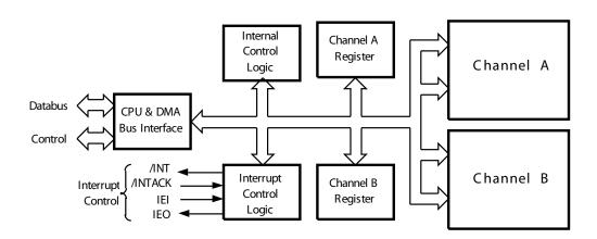
Figure 1. Z85233 Functional Block Diagram
