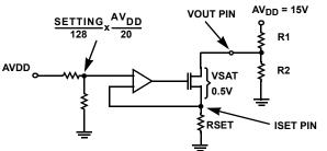
FIGURE 5. OUTPUT CONNECTION CIRCUIT EXAMPLE
