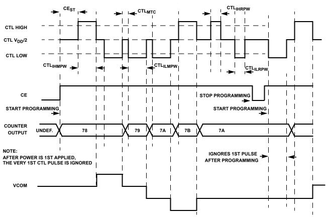
THE TIMING DIAGRAM ABOVE SHOWS POST POWER-UP TIMING.
