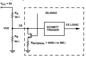
FIGURE 7. APPLICATION GENERATING VDD AND VCE VOLTAGES
