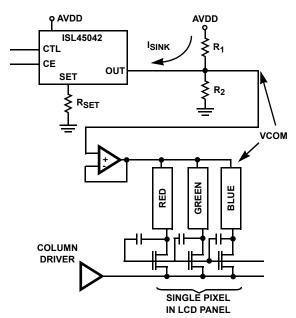
FIGURE 1. VCOM ADJUSTMENT IN AN LCD PANEL
