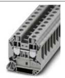
Feed-through terminal block, Connection method: Screw connection, Cross section: 1.5 mm<sup>2</sup> - 25 mm<sup>2</sup>, AWG: 16 - 4, Width: 12.2 mm, Height: 54.4 mm, Color: black, Mounting type: NS 35/7,5, NS 35/15
