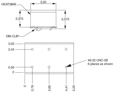
DIMENSIONS: inches TOLERANCES: ±0.02 inches MATERIAL: AISI 6063-T5 Aluminum FINISH: Black Anodized
