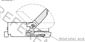
3. The actuator will not open more than 135°. Do not apply any force backward beyond this point. Otherwise, the actuator may come off or break.
