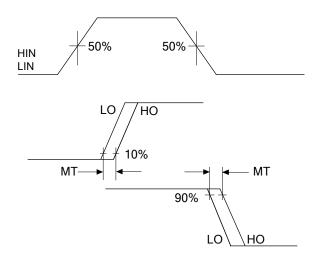
Figure 3. Delay Matching Waveform Definitions
