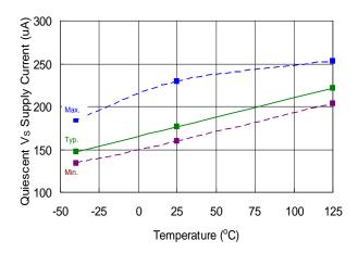
Figure 13. V<sub>BS</sub> = 18V Supply Current vs. Temperature
