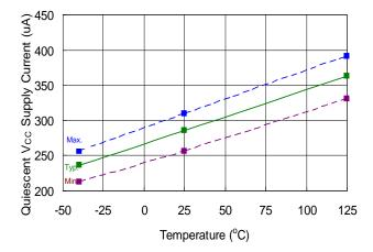
Figure 12. V<sub>CC</sub> = 18V Supply Current vs. Temperature
