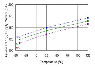
Figure 10. V<sub>CC</sub> Supply Current vs. Temperature
