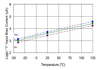
Figure 16. Logic "1" Input Bias Current vs. Temperature
