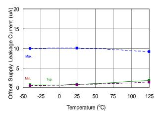
Figure 9. Offset Supply Current vs. Temperature
