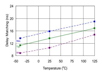
Figure 8. Delay Matching Time vs. Temperature
