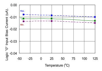
Figure 17. Logic "0" Input Bias Current vs. Temperature
