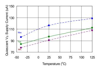
Figure 11. V<sub>BS</sub> Supply Current vs. Temperature
