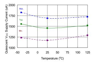
Figure 14. V<sub>CC</sub> = 20V Supply Current vs. Temperature
