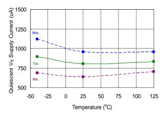
Figure 15. V<sub>BS</sub> = 20V Supply Current vs. Temperature
