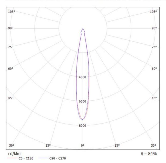
Luminaire: LEDiL Oy CN13188\_LENA-M\_(CXA1520) Lamps: 1 x CREE\_CXA1520\_(CXA1520-30F-N4-N0H-0001)\_972.29@250mA\_CCT=3000K\_P=8.22841W\_I=249.8mA
