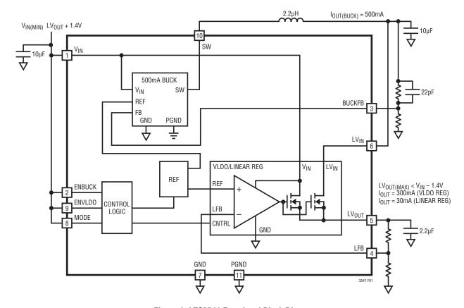
Figure 1. LTC3541 Functional Block Diagram
