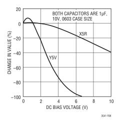
Figure 8. Change in Capacitor vs Bias Voltage
