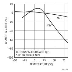
Figure 9. Change in Capacitor vs Temperature
