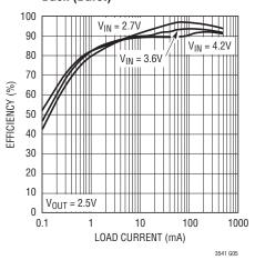
Efficiency vs Load Current for Buck (Pulse Skip)
