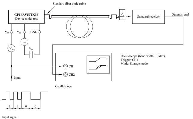
Fig. 4 Input Signal (6.6 Mb/s Bi-phase PRBS Signal)
