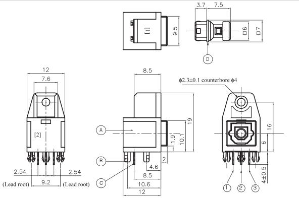
Example of mounting drawing from solder side.
