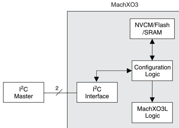
There are two hardened I<sup>2</sup>C controllers in a MachXO3L/LF device, a primary and a secondary. The primary controller provides an interface to the MachXO3L/LF Configuration Logic. The primary I<sup>2</sup>C controller is the only one that permits access to the Configuration Logic OR can be a User Mode I<sup>2</sup>C controller. The Secondary I<sup>2</sup>C controller is always a User Mode I<sup>2</sup>C controller.
