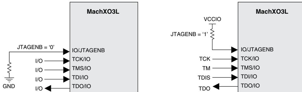
It is critical when using the JTAGENB feature that logic attached to the JTAG I/O pins not contend with a JTAG programming system. The external logic must ignore any JTAG transactions performed by an external programming system.
