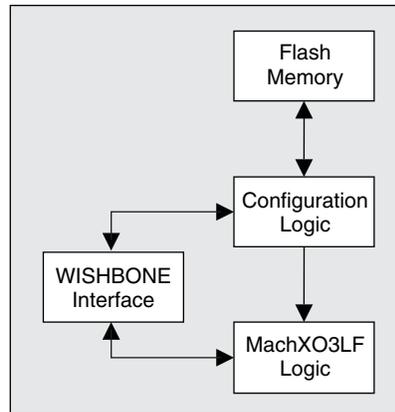
The MachXO3LF must be in user mode in order to access the WISHBONE interface. Accessing and updating the resources made available by the configuration logic must be done in Transparent mode. Attempting accesses to the configuration logic in offline mode causes a deadlock because the MachXO3LF leaves user mode.
