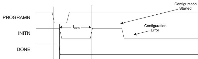
The INITN pin of a MachXO3L device is not visible external to the device when in the Feature Row HW Default Mode state. The INITN pin, when in this mode, is pulled high by default. The INITN behavior described in Figure 7 is only visible outside the MachXO3L when the INITN pin is enabled.
