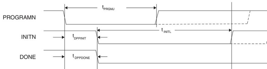
**INITN:** The INITN pin is a bidirectional open-drain control pin. It has the following functions:
