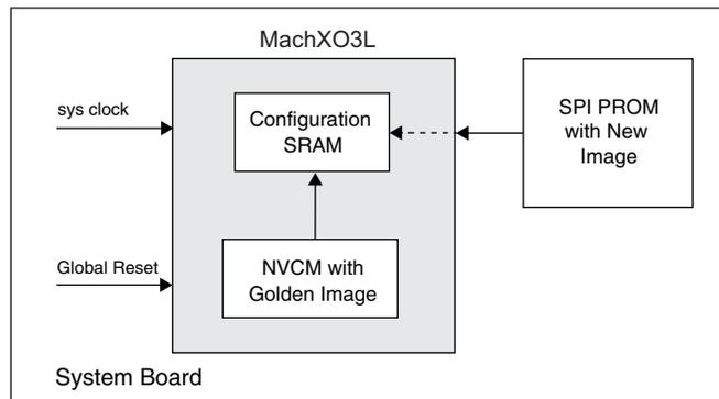
The example assumes that you have the golden image stored in NVCM in order to initiate the system, and will then use SPI PROM as a resource for image updates without disturbing the system. Figure 16 shows the process flow for performing this task.
