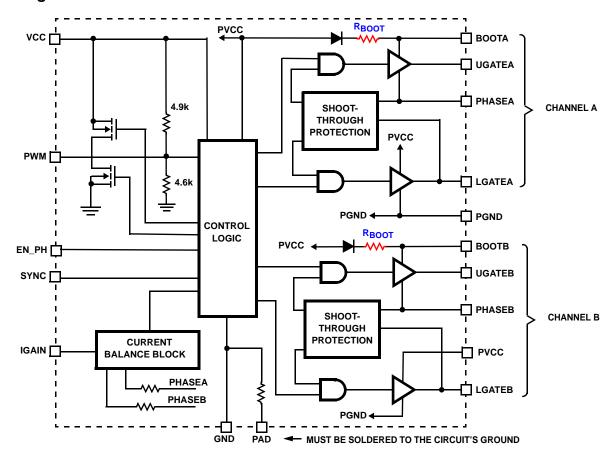
INTEGRATED 3 $\Omega$  RESISTOR (RBOOT) IN ISL6611A
