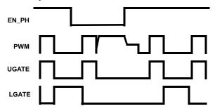
FIGURE 5. TYPICAL EN\_PH OPERATION TIMING DIAGRAM
